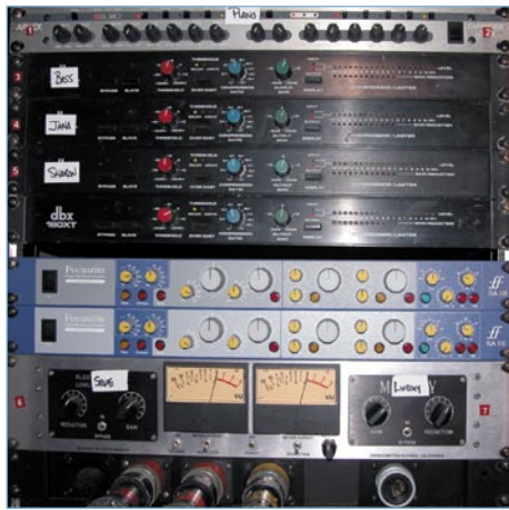
Rack of compression: (From top) Aphex Expander/Gate, 4 x dbx 160X compressors, 2 x Focusrite mic preamp/EQ, while the Manley electro-optical compressor was used for Stevie Nicks' and Lindsay Buckingham's vocals.
