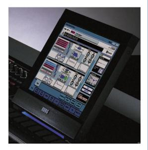
40GB drive as WAV files in 16-bit/48k format at anything up to 80 minutes in length. Each track is automatable for volume, pan, EQ and effect sends with a song region limit of 5,000 clips. Why Korg didn't go the full monty and provide 24-bit file recording is a mystery. But, suffice it to say, recording at 16-bit via any of the microphone emulations sounds more than adequate.
